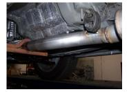
3. Install headpipe #A onto your existing stock front pipe and secure using clamp #G. Use a jack stand to support the converter. Insert welded hanger into rubber grommet.
