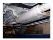
4. Install muffler #B onto headpipe #A 1.5-2" with the louvers facing towards the converter. Use a jack stand to support the muffler. Use clamp #H to secure the muffler to the headpipe. Do not tighten. Muffler inlet is looking into the louvers.
