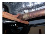
2. To remove the stock exhaust, unclamp it at the connection in front of the stock muffler. Disengage the welded hangers from the rubber grommets using WD-40 to aid in this process. Do not damage or remove the rubber grommets as you will re-use them to mount the new system.
